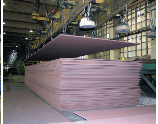
UNLOADING FINISHED, COATED PLATE.
