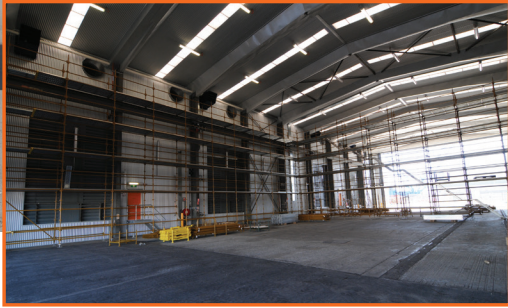
A TYPICAL LARGE BLAST AND PAINT HALL FOR SHIP SECTIONS: 75 FEET WIDE X 45 FEET HIGH X 180 FEET LONG
